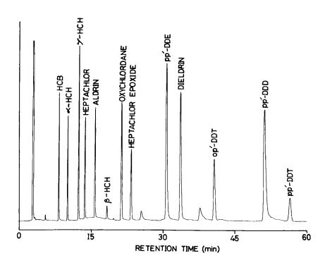
Figure 1. Standard chromatogram with major peaks of different OCI as per their retention time. Perkin Elmer VIT silica capillary column containing 25 QCZ/OV 1701, length-25 m, id-0.2 mm; carrier gas, argon/methane (90/10) at 15 PSIG; injection port temp, 220°C; detector temp, 275°C; column temp, 215°C; chart speed, 2 cm/min.
